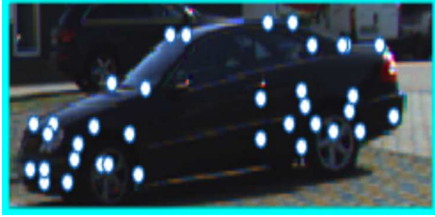
Figure 3.5 This figure shows the 36 keypoints used in our shape representation. The projections of the semantic keypoints are displayed using white circular markers. These semantic keypoints have been carefully chosen to capture adequate variance in the shapes of cars.
