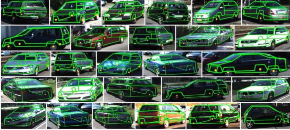
Figure 3.8 A collage of different types of cars with the corresponding wireframe overlaid on them. The wireframes were generated by connecting the detected keypoints by the proposed stacked hourglass network
