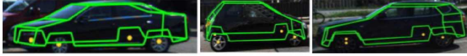
Figure 3.3 In this figure we see the capability of the chosen 36 keypoints to adequately model different class of cars – sedan, hatchback, and an SUV. For a better illustration, the keypoints have been connected based on their order to form a wireframe in green color.
